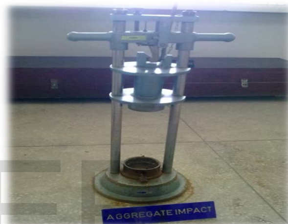
FIGURE 2: Aggregate Impact Value Apparatus
